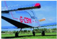
Eurostar is very low to the ground which aids exit and entry; prop clearance good for rougher fields
