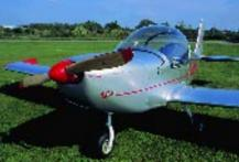
Closely coweled nose hides 80hp Rotax 912, perfectly adequate power for such a lightweight
