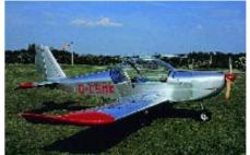
Thin anodised aluminium skin is traditionally manufactured; the lack of paint saves weight
