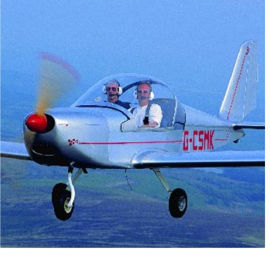
127kt. At about this point in a Dyn'Aero Ban-bi I had experienced a pitch oscillation through the stick which I found alarming. Not here. The Eurostar's little trim lever, which sits between the two seats, came in handy as the out-of-trim forces began to build. At this point the controls still felt great, and not heavy in roll or sensitive in pitch as with some others.
